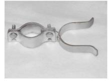
Heavy pressed steel forks are 8 gauge x 1" fittings that along with gate collars form a fork latch assembly. The heavy fork comes in six sizes for post sizes ranging from 1 7/8" to 3".
