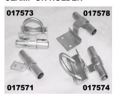
Clamps on with brace bands or u-bolts depending on style. Will fit 2 3/8" or 2 7/8" pipe. Can also fit 2" if specified using smaller U-bolt. Holders designed to clamp rolling gate track tubing onto fence so that fence gate will bypass existing fence. Available in several styles to meet your entire gate hanging needs. Also referred to as gate track brackets.
