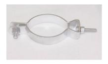
13 gauge x 1" steel strip designed to mount signs to 2 3/8" steel post. This bracket comes with 2 - 5/16" x 1 1/4" carriage bolts and is an inexpensive sign bracket to install commercial signage.
