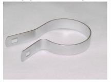
Tension bands are an offset strip of metal shaped to fit around the terminal post and used with a carriage bolt and nut to attach the tension bar to the post. These bands are made from 11 gauge x 1" steel. This gauge band is used in heavy-duty commercial applications. A 3/8" x 1 1/2" carriage bolt is used. Carriage bolt and nut sold separately.
