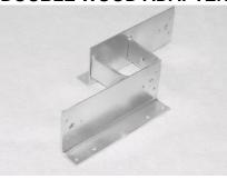
14 gauge brackets used when double-sided fence is required. Made from 14 gauge steel with 9 gauge strap for pipe attachment with set screw and lip.
