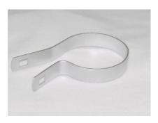
Tension bands are an offset strip of metal shaped to fit around the terminal post and used with a carriage bolt and nut to attach the tension bar to the post. These bands are made from 14 gauge x 3/4" steel. This gauge band is used in residential and other light duty applications. A 5/16" x 1 1/4" carriage bolt is used. Carriage bolt and nut sold separately.
