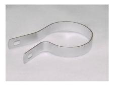
Tension bands are an offset strip of metal shaped to fit around the terminal post and used with a carriage bolt and nut to attach the tension bar to the post. These bands are made from 13 gauge x 7/8" steel. This gauge band is used in medium duty applications. A 5/16" x 1 1/4" carriage bolt is used. Carriage bolt and nut sold separately.
