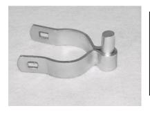
Post hinges are a fitting that attaches to the gatepost, the pintle of which fits the frame hinge permitting the gate to swing. These hinges are made from 8 gauge x 1 1/4" wide or 8 gauge x 1 1/2" wide steel. A 3/8" x 2" through 3 1/2" carriage bolt and nut are used. Carriage bolt and nut sold separately.
