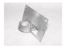
14 gauge flat bracket with holes at all four corners, designed to fit any post from 1 3/8" to 4 1/2" by using proper brace band for attachment. Design features smooth backside of post. Band, bolt and nut sold separately.
