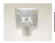
Wall mount hinges are a swing gate hinge that permits the gate to swing 90° from the closed to open position. The flat plate is mounted to a wall or flat surface and can be used on 1 5/8" or 1 7/8" gate frames.
