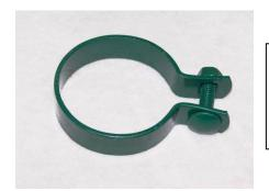
12 gauge x 3/4" strip of metal shaped to fit around post to attach rail ends to that post. Can also be used to attach tighteners, brace rail ends or barbwire to post. A 5/16" x 1 1/2" carriage bolt and nut is included.
