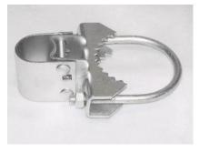
Pressed steel bulldog hinges are a swing gate hinge that permits the gate to swing 90° from the closed to the open position. Bulldog hinges are attached to the post with a 1/2" U-bolt.
