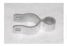
Female gate hinges are a fitting that attaches to the gate frame and functions with the post hinge (also called frame hinge). A 3/8" carriage bolt is used. Carriage bolt and nut sold separately.
