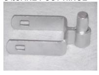
Square post hinges are a fitting that attaches to the gate post, the pintle of which fits the frame hinge permitting the gate to swing. A 3/8" x 1 1/2" through 4 1/2" carriage bolt and nut is used. Carriage bolt and nut sold separately. 9 gauge.
