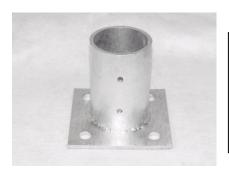
6" x 6" x 1/4" steel flanges with 5/8" holes at each corner. Has 5 1/4" tall flange with 2 set screws to secure tubing. Available for 2", 2 1/2", 3" tubing. The 4" tubing is on a 8x8x1/4" plate. Our galvanized flanges are 1/4" thick. Used for many job start scenarios involving anchoring steel tubing to flat surfaces.
