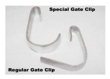
Gate clips are 12 gauge steel fittings used to attach gate fabric to the vertical sides of a gate frame.
