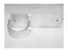
End of line wood adapter for attaching wood rails to steel posts. Made from 14 gauge steel with 9 gauge strap with set screw. Has 90° lip for wood rail support.
