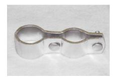
Split kennel hinges are a fitting that one half of the hinge allows the kennel gate frame to swing while the other half attaches to the kennel panel. Two 3/8" x 1 1/2" carriage bolts and nuts are used. Carriage bolts and nuts are sold separately. 8 gauge x 1 1/2" material.
