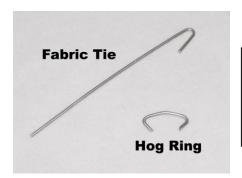
Fabric ties designed to attach chain link to rail tubing. Steel ties are available in 12 gauge with different lengths. Aluminum ties are available in 9 and 11 1/2 gauge with different lengths. Pig rings are 12 gauge steel and come in 10 lb. boxes.
