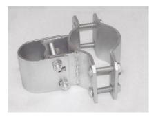
Pressed steel box hinges are a swing gate hinge that permits the gate to swing 90° from the closed to the open position. Box hinges are attached to the post with a strap and four 3/8" carriage bolts. Carriage bolts and nuts are included.
