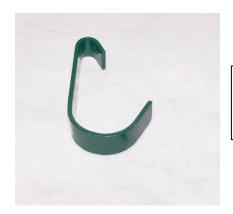
Gate clip designed to be installed with special gate clip tool, to attach fence fabric to gate frame. Used on sides of gate frame in conjunction with tension bars.
