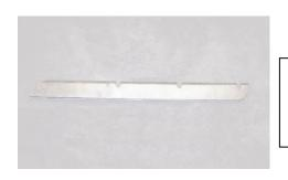
Three wire clamp-on barbed wire extension arms are made of pressed steel and are attached to the post with brace bands. These arms are 18" long and 14 gauge.
