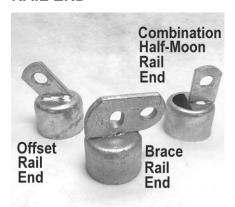
Offset rail ends are a cup-shaped fitting used with a brace band, carriage bolt and nut to connect the top rail or brace to a post. Carriage bolt and nut sold separately. These have 1 hole and the tab is fastened to top of cup at a 45°. **F** = **Import**
