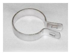
Brace bands are a symmetrically formed strip of metal shaped to fit around a post and used with a carriage bolt and nut to attach the rail end or brace rail end and truss rod tightener to the post. Also used for attaching barbed wire, tension wire, and other items to a terminal post. These bands are made from 13 gauge x 7/8" steel. This gauge band is used in residential and other light duty applications. A 5/16" x 1 1/4" carriage bolt is used. Carriage bolt and nut sold separately.
