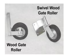
Rollers designed for wood gates. Available for lag screwing to gate rails, in either fixed or swivel configurations. Uses 6" solid rubber tires. Swivel gate roller uses 4" x 4" x 1/8" plate with 4 holes for sturdy mounting.
