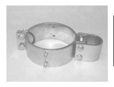
Pressed steel box hinges are a swing gate hinge that permits the gate to swing 90° from the closed to the open position. Hinge is attached to the post with a strap and four carriage bolts. Carriage bolts and nuts are included.
