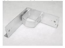
90° bracket to attach wood rails to corner steel posts. Bracket is 14 gauge and strap is 9 gauge galvanized metal with set screw. Has 90° lip on adapter for rail to
