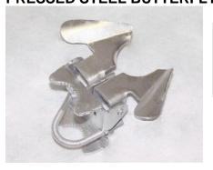
A gate fitting used to hold a gate in place when closed. Used on 1 3/8" gate frame with two fork sizes of 1 7/8" & 2 3/8". Has padlock hole under latch to secure gate. **Import**
