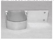
Heavy 3/16" x 2" steel bracket with 9 gauge strap with set screw designed to be used at the end of the line. Used same as above but without a lip so that you can attach it to any flat surface.
