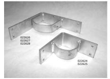
Bracket designed for inside corner applications. Made of 3/16" x 2" steel with 9 gauge strap with set screw. Does not have lip, so can be mounted on any flat surface.
