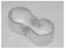
Panel clamps are a two-piece clamp designed to secure prefabricated panels on freestanding enclosures. These clamps are made from 8 gauge x 1 1/2" wide steel with approximately 1/2" spacing between the two pieces of tubing. Carriage bolt and nut sold separately.
