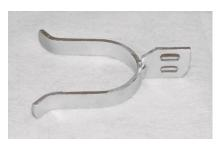
Heavy pressed steel forks are 8 gauge x 1" fittings that along with gate collars form a fork latch assembly. The heavy fork comes in six sizes for post sizes ranging from 1 5/8" to 4". Sizes 3 1/2" and 4" are 8 gauge x 1 1/4"
