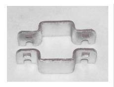
Square gate collars are used with square tubing in ornamental fencing to attach to a gate fork and square post with carriage bolts to form a gate latch assembly. The collars are made with 8 gauge steel and come in four sizes:
