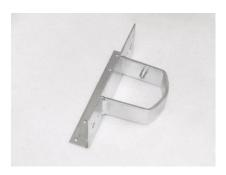
14-gauge steel-ell bracket with 9-gauge strap with set screw. Designed to screw onto wood rail and be supported by steel fence post. Very popular item to run wood fencing using steel posts.
