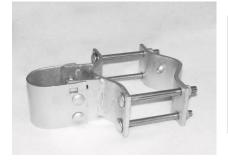
Universal pressed steel box hinges are a swing gate hinge that permits the gate to swing 90° from the closed to the open position. Universal box hinges are attached to the post with a strap and four 3/8" carriage bolts. These hinges are universal because they fit post sizes 2 1/2" through 4 1/2". Bolts and nuts included.
