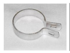
Brace bands are a symmetrically formed strip of metal shaped to fit around a post and used with a carriage bolt and nut to attach the rail end or brace rail end and truss rod tightener to the post. Also used for attaching barbed wire, tension wire, and other items to a terminal post. These bands are made from 12 gauge x 3/4" steel. This gauge band is used in residential and other light duty applications. A 5/16" x 1 1/4" carriage bolt is used. Carriage bolt and nut sold separately.
