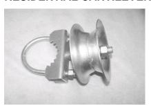
1 5/8" roller assembly with U-bolt for 2 7/8" tubing. Can also make for 2 3/8" and 4". Designed for light residential use. Uses a pressed steel roller and has sealed bearing assemblies.
