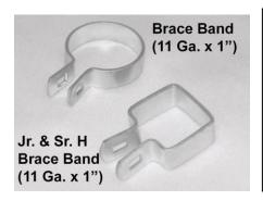
Brace bands are a symmetrically formed strip of metal shaped to fit around a post and used with a carriage bolt and nut to attach the rail end or brace rail end truss and rod tightener to the post. Also used for attaching barbed wire, tension wire, and other items to a terminal post. These bands are made from 11 gauge x 1" steel. This gauge band is used in heavy-duty commercial applications. A 3/8" x 1 1/2" carriage bolt is used. Carriage bolt and nut sold separately.
