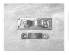
Line wood adapter for 2 3/8" steel posts. Bracket is 13ga. X 2" X 6", and strap is 13ga. X 7/8". Designed to use 2 - 5/16" X 1  $\frac{3}{4}$ " carriage bolts (not included). Bracket has 4 holes for rail attachment.
