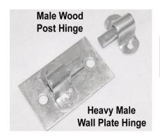
Male post hinges made in 8 gauge galvanized steel and have 5/8" pins. Heavy male hinge uses 3" x 5" plate for attachment.
