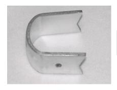
Used to weld to pipe for running rail, either 1 5/8" or 1 7/8" size. 9 gauge material.
