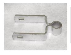
Female gate hinges are a fitting that attaches to the gate frame and functions with the post hinge (also called frame hinge). Square female gate hinges are used in applications where square gate frames are used such as ornamental fence. A 3/8" carriage bolt is used. Carriage bolt and nut sold separately. 8 gauge.
