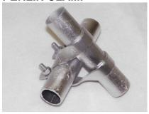
12 gauge x 3/4" 2 piece strap steel clamp designed to join two pipes at 90° angles. Used mainly in the construction of greenhouses, but can also be used to build portable buildings and for many other uses. Strap steel which is twisted and galvanized, are sold without bolts.
