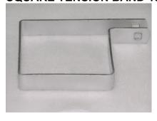
Tension bands are an offset strip of metal shaped to fit around the terminal post and used with a carriage bolt and nut to attach the tension bar to the post. These bands are made from 13 gauge x 7/8" steel. Square bands are used in applications where square posts are used such as ornamental fence. A 5/16" x 1 1/4" carriage bolt is used. Carriage bolt and nut sold separately.
