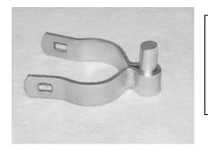
Post hinges are a fitting that attaches to the gatepost, the pintle of which fits the frame hinge permitting the gate to swing (also called male hinge). These hinges are made from 8 gauge x 1" wide steel. A 3/8" x 1 1/2" through 3 1/2" carriage bolt is used. Carriage bolt and nut are sold separately.
