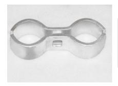
Saddle clamps are a two-piece clamp designed to secure prefabricated panels on freestanding enclosures. These clamps are made from 7 gauge x 1" wide steel with approximately 1 1/4" spacing between the two pieces of tubing. Carriage bolt and nut sold separately.
