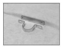
Welded Wire Clamps are designed to attach welded wire panels to the post for support of your panels. Available in 1 5/8", 1 7/8", 2 3/8", 2 7/8" and 4" sizes. Material is 11 gauge x 1.
