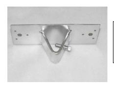
14 gauge pressed steel bracket designed to hold rails when building fence using T-post. Has lip on bottom and set screw digs into "T" on post for secure fastening.
