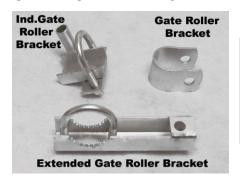
Gate roller brackets are designed to connect the gate roller to the gate for tracking purposes. They are available for 1 3/8", 1 5/8" and 1 7/8" tubing sizes. Also in industrial and extended sizes for special uses. They can be bolted on with U-bolts or single bolts.
